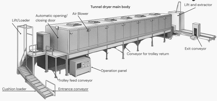
A drying tunnel has to perform day in and day out, but what keeps production moving isn't just airflow and temperature control, it's how easily the system can be maintained. For engineers and plant managers, downtime is the hidden cost that can dwarf energy savings if the tunnel isn't designed for access and service.
