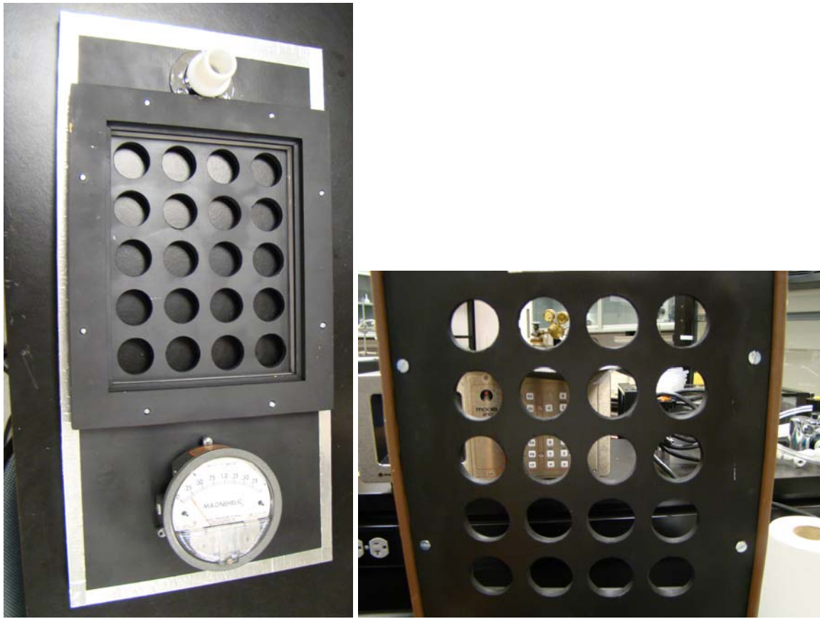
Figure 3. Make up air entry with magnehelic gauge, aerosol entry port, weather stripping
