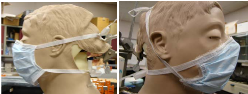
Figure 27. Unsealed Cobeal mask under normal use Figure 28. Sealed mask with crossed straps
