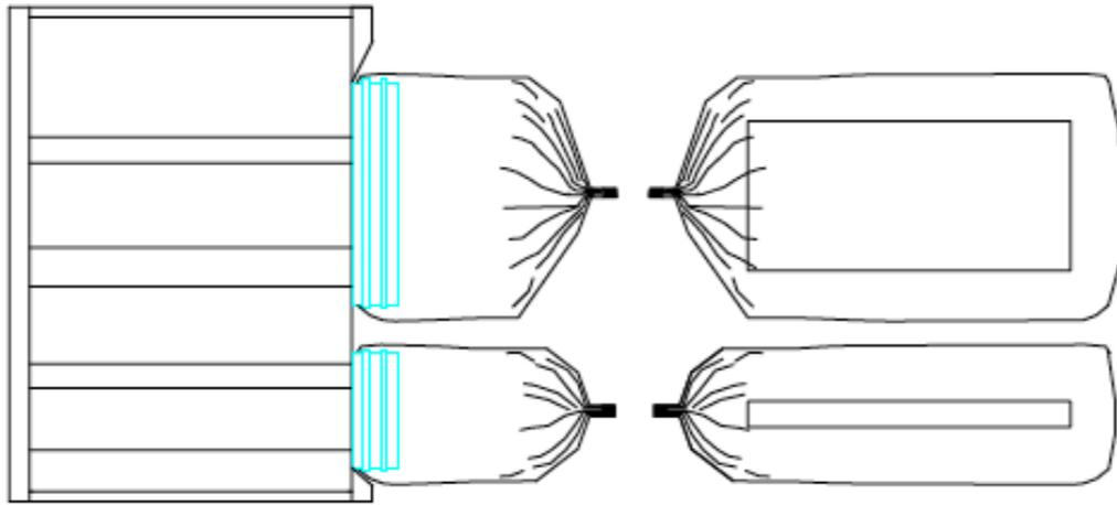
Top view of both a pre-filter and HEPA filter change out-sealing lip in blue
