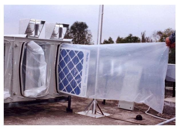
Cobeal's BIBO filter housings for fluid or gasket seal primary filters are side-loading filter housings which have been designed to meet the air filtration needs of industries and research facilities that handle dangerous, toxic, biological or carcinogenic material. To minimize exposure to harmful contamination while replacing used filters, the housing incorporates a ribbed BIBO ring, over which a heavy-duty plastic filter bag is attached (see left).
