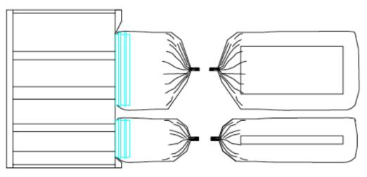
Top view of both a pre-filter and HEPA filter change out-sealing lip in blue
