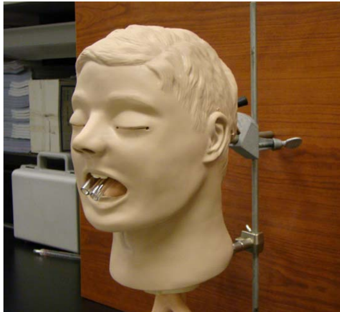
Figure 9. Manikin head on mounting bracket
