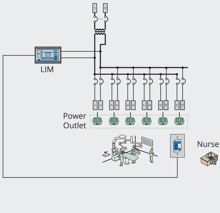
**With a basic isolated power system, the procedure is the following in case of fault:**
