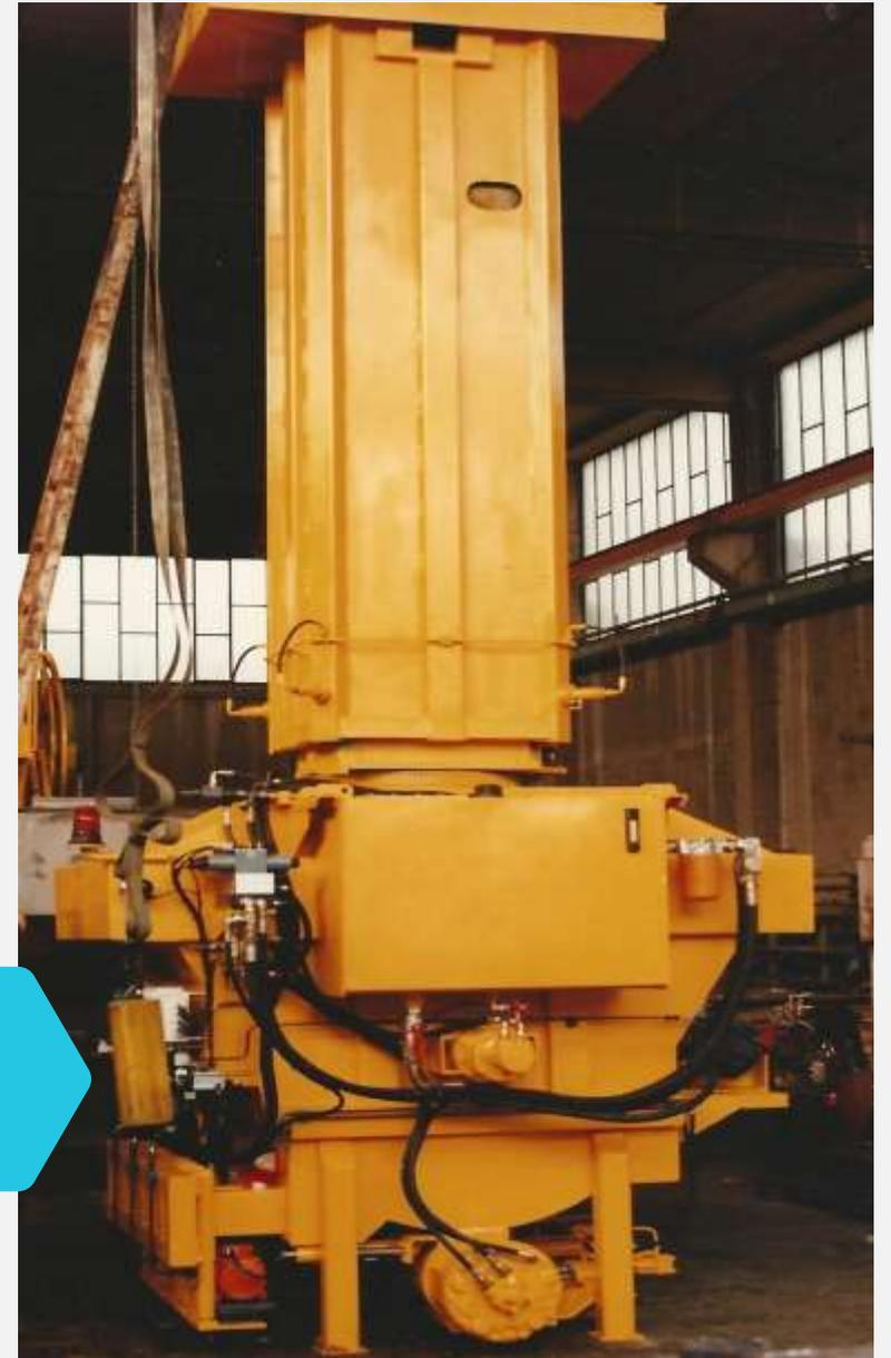
Machine can spread and screed from 0.1 to 1 cubic meter (1.3 cyd) per min with slump from 0 to 250 mm (0 to 10")
