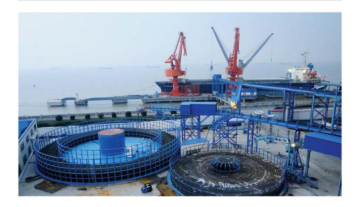
Submarine power cable are used for interconnection of offshore power fields, tidal wave locale, wind mill and offshore oil & gas platforms and also islands. The voltage for such application are usually less than 36kV AC type and typically uses the 3cores XLPE cables.
