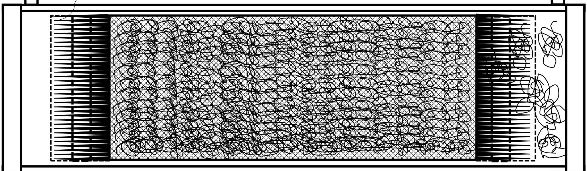
Harvest trolley could be symmetric and travel in both directions (without needing to be rotated), between trucks on both ends of raceway. After harvesting from one festoon, the harvest trolley would empty collected gracilaria into one of said trucks before being launched into a new festoon traveling in the opposite direction back towards the other truck.
