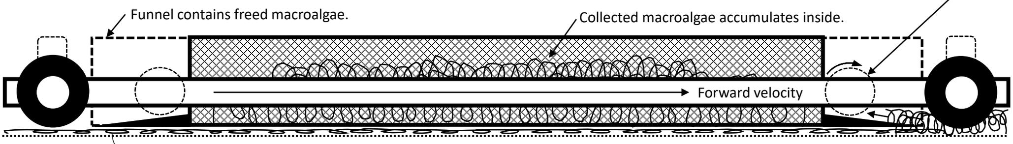
Harvester could leave a thin layer of macroalgae to allow further growth, or completely clean the mesh (so that it can be re-seeded).
