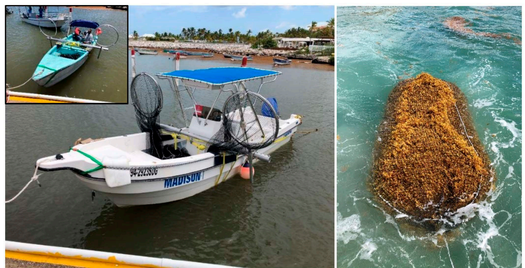
Figure 2. (Top Left) Littoral Collection Module (LCM) fitted onto a traditional “yola” boat. (Left) LCM fitted onto a small powerboat prior to the arms rotating the nets down into the water. (Right) A net of Sargassum filled by the LCM, floating in the water before it is towed away.
