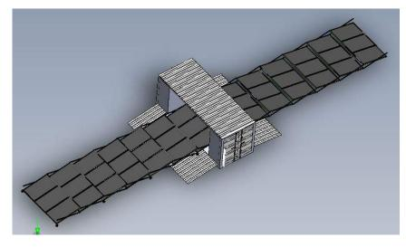
REAR CABIN: DIESEL GENERATOR MIDDLE CABIN: PV PANELS FRONT CABIN: BATTERY AND INVERTER GROUP
