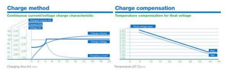
The prefered charging procedure should be in accordance with DIN 41773, constant current/constant voltage (U characteristic). Constant foat charging utilizing a constant voltage charger is also acceptable.
