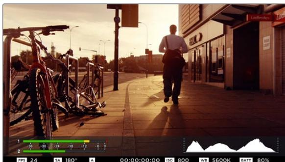
In Blackmagic Micro Cinema Camera, the status strip and on screen meters can be viewed on the HDMI or composite output display.
