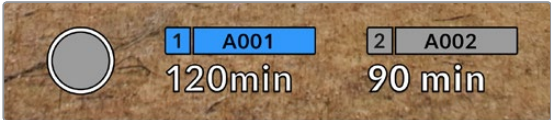
Your URSA Mini's storage indicator will display the name of your CFast card, SD card or SSD and the record time remaining in minutes
