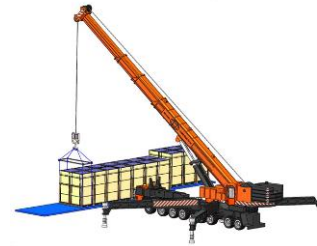
Long-side vertical package unloading with crane
