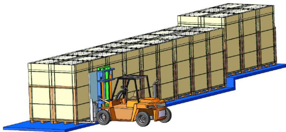
Long-side vertical package unloading with forklift
