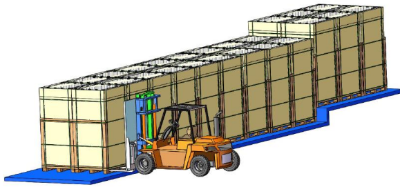
Long-side vertical package unloading with forklift
