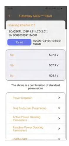
On the site details page, click on the target device in the device list to enter the detailed data and settings page for the specific device.
