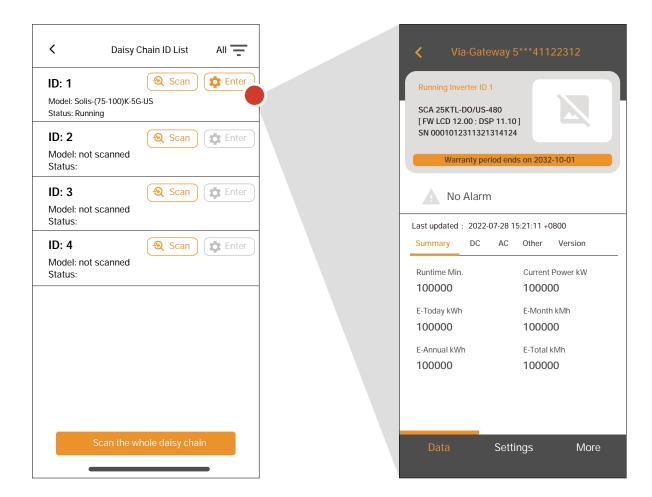
Click "Device Settings" to view the inverter data. If the inverter needs to be initialized, the APP will prompt to set parameters such as grid code or clock.
