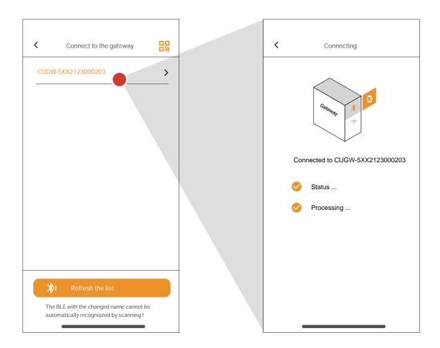
The gateway SN is included in the BLE signal name, and the app will list the scanned signals. Select the SN consistent with the target gateway label and click to enter.
