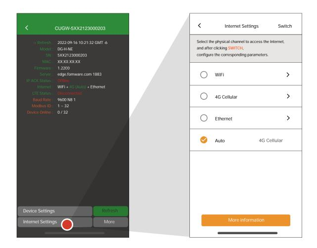
Ensuring that the gateway can connect to the Internet is the most important step.
