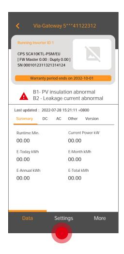
The APP logs in to the inverter setting interface through BLE.
