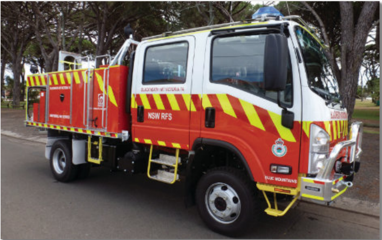
A Category 7 firefighting vehicle (Image by Soil Conservation Service's NSW RFS Fire Trail Manual)
