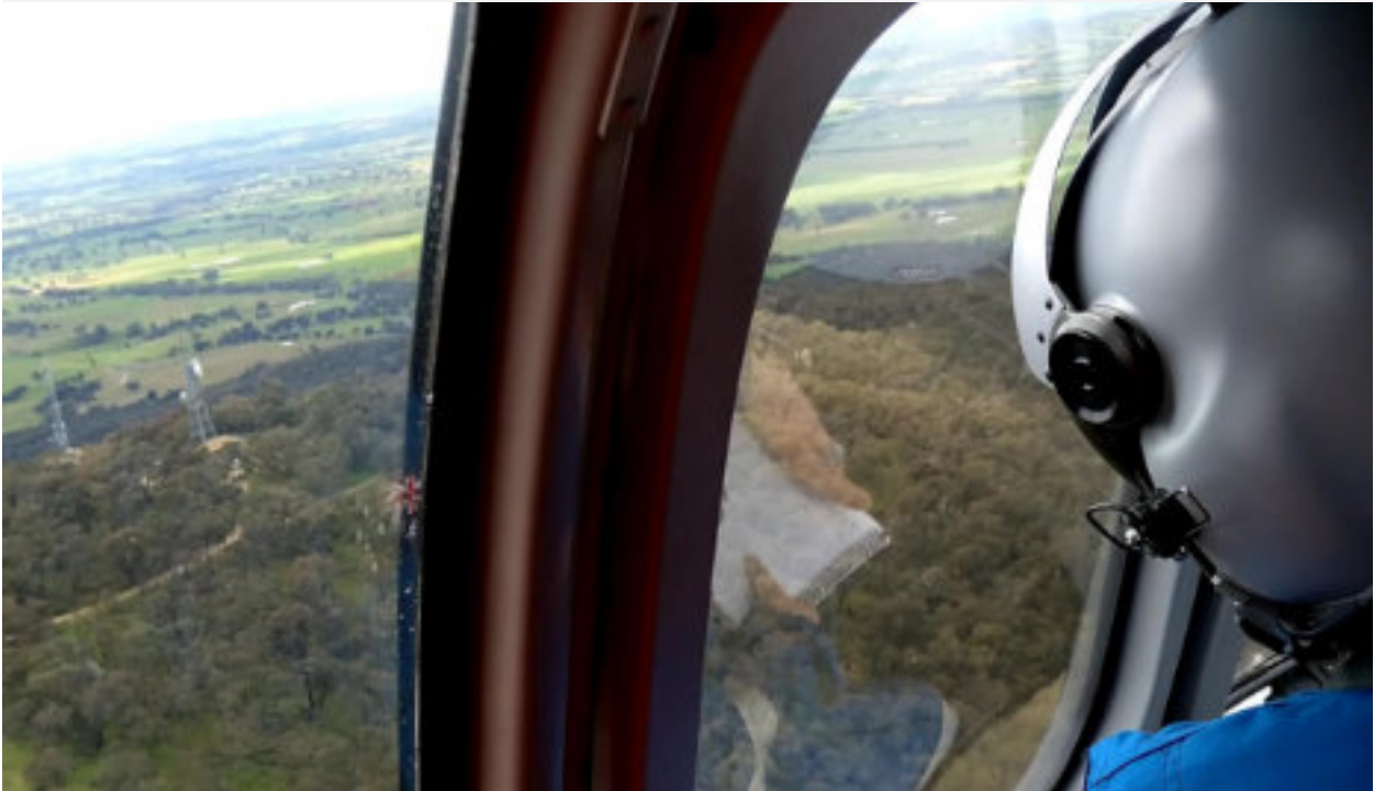
During the low-flying aerial inspection phase, the aircraft must be flown at an altitude commensurate with the environmental visibility and that of the target. Likely areas for turbulence must be identified and all crew members must be vigilant for hazards, especially in their arcs of visual responsibility. (Image by Conway Bown)
