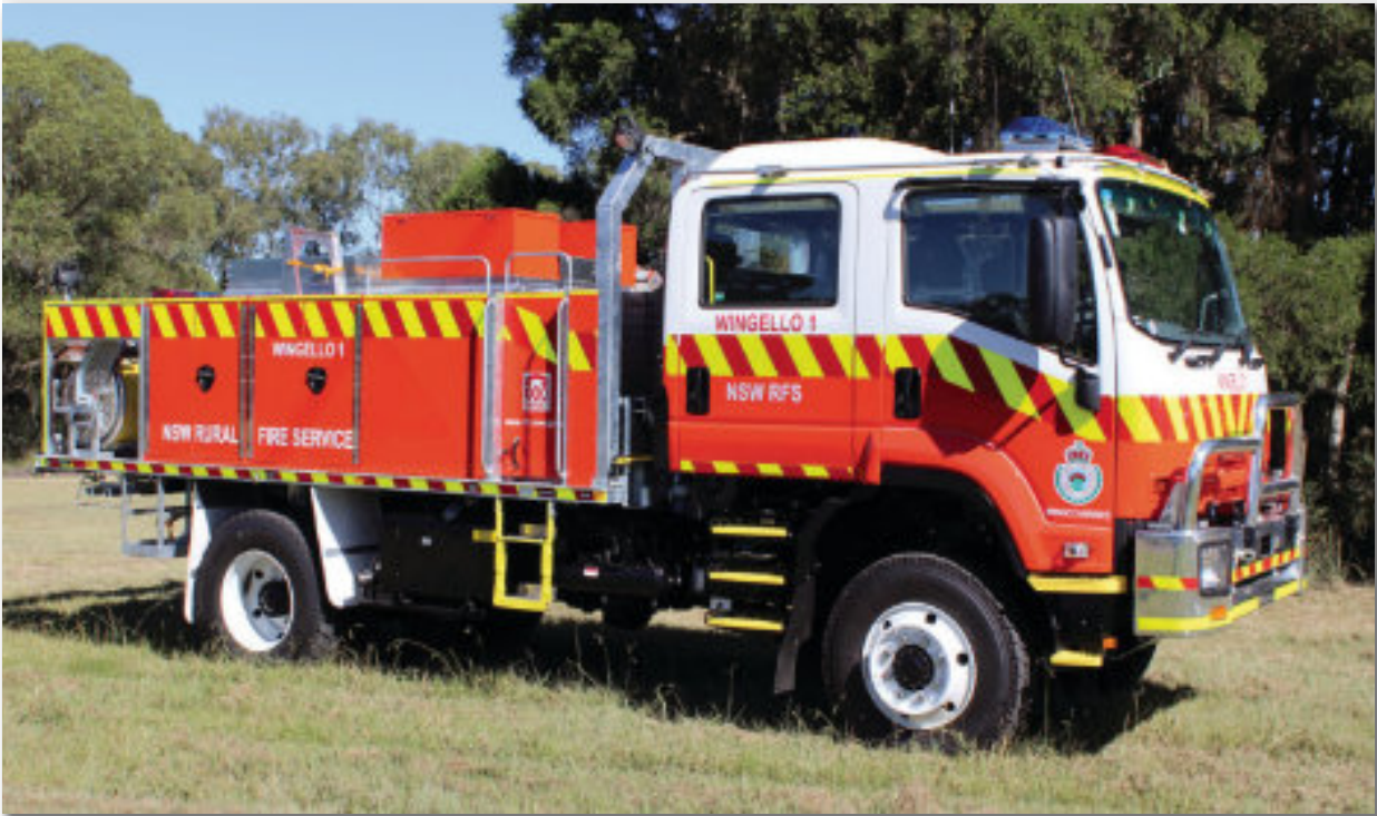
A Category 1 firefighting vehicle (Image by Soil Conservation Service's NSW RFS Fire Trail Manual)
