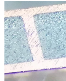
Self-developed copper plating additives and THP through-hole plating effect
