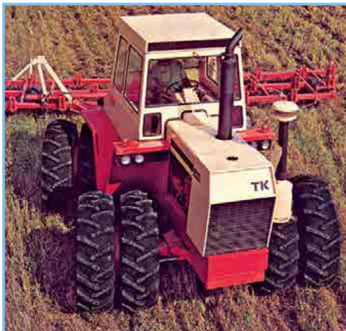
The Case 1470 provided the operator the choice of coordinated front and rear steering, crab steering, front steering, or rear steering.
