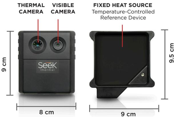
Seek Scan™ is a simple, low-cost, thermal imaging system designed to automate body temperature screening using skin temperature as a proxy. With  $\pm 0.3^{\circ}\text{C}$  ( $\pm 0.5^{\circ}\text{F}$ ) accuracy and the inclusion of a reference heat source, Seek Scan delivers the same performance as an infrared temporal thermometer - but with a safe social distance.
