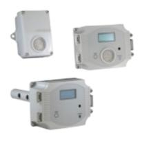
The AZ-CMD Series carbon monoxide detector uses an electro-chemical sensor to monitor the carbon monoxide level and out-puts a field-selectable 4-20 mA, 0-5 or 0-10 Vdc. The sensing range and output may be scaled to either 100, 150, 300, 400 or 500 ppm via the on-board menu. A front panel LCD is standard to ensure easy setup and operation. It is available in either wall/surface or duct mount configurations.
