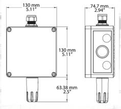
The horticulture sensor can be mounted directly onto any wall or flat surface, or may be suspended from the ceiling using the device cable harness which is secured to the enclosure with a compression style fitting.
