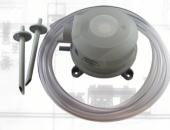
**AZC-GDT** differential pressure switch unit contains a snap-acting SPDT switch, and a range adjustment knob with increments. The sample connections located on the side accept 6.35mm (0.25") OD tubing. There are various optional pressure ranges, and 2 pickup tubes and 6 ft of PVC tubing included.
