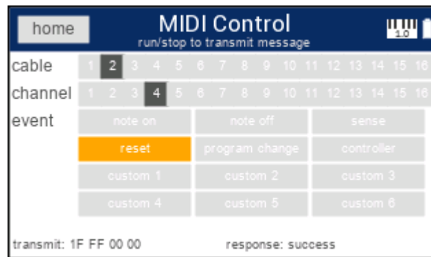
Example MIDI reset message sent on cable 2
