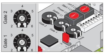
The gate leaf length is set with the "Gate 1" (M1/gate leaf with stop) + "Gate 2" (M2/gate leaf with walk-through gate) potentiometers.
