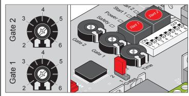
The length of the gate leaf is set at the control unit with the "Gate 1 (M1) + Gate 2 (M2)" potentiometers. The speed of movement and the force tolerance for the separate leaves of the gate installation are determined based this setting.
