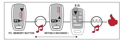
The receiver checks the incoming remote signal is the correct encoding before forwarding the command. Thus, the remote button has to be pressed for approx. 1–2 seconds duration.
