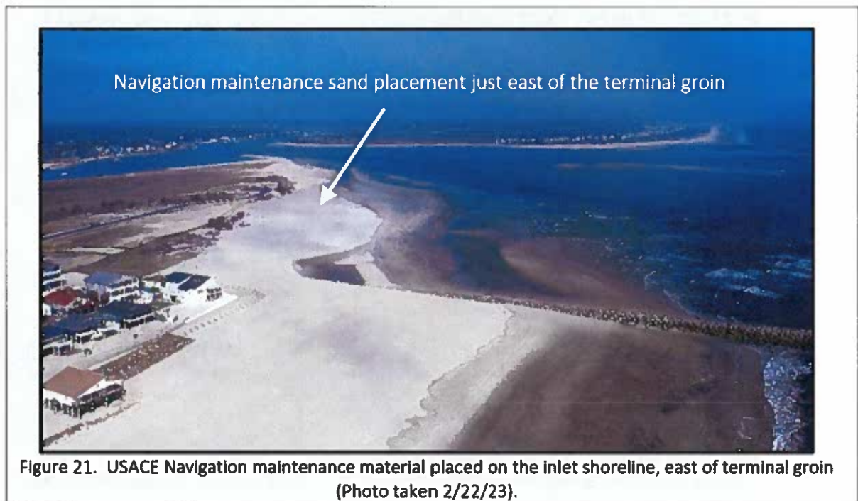
Figure 3-10. Excerpted photo from April 2024 Ocean Isle Beach Terminal Groin monitoring report. Placement of the 2023 Shallotte Inlet crossing sand was downdrift of the terminal groin.
