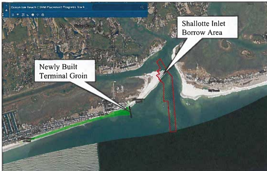
Figure 3-9. Ocean Isle Beach 2021/2022 Terminal Groin and Federal CSRM Beach Renourishment Projects. Shallotte Inlet Borrow Area and Placement Area Shown (USACE Ocean Isle Beach CSRM Placement Progress Tracker)
