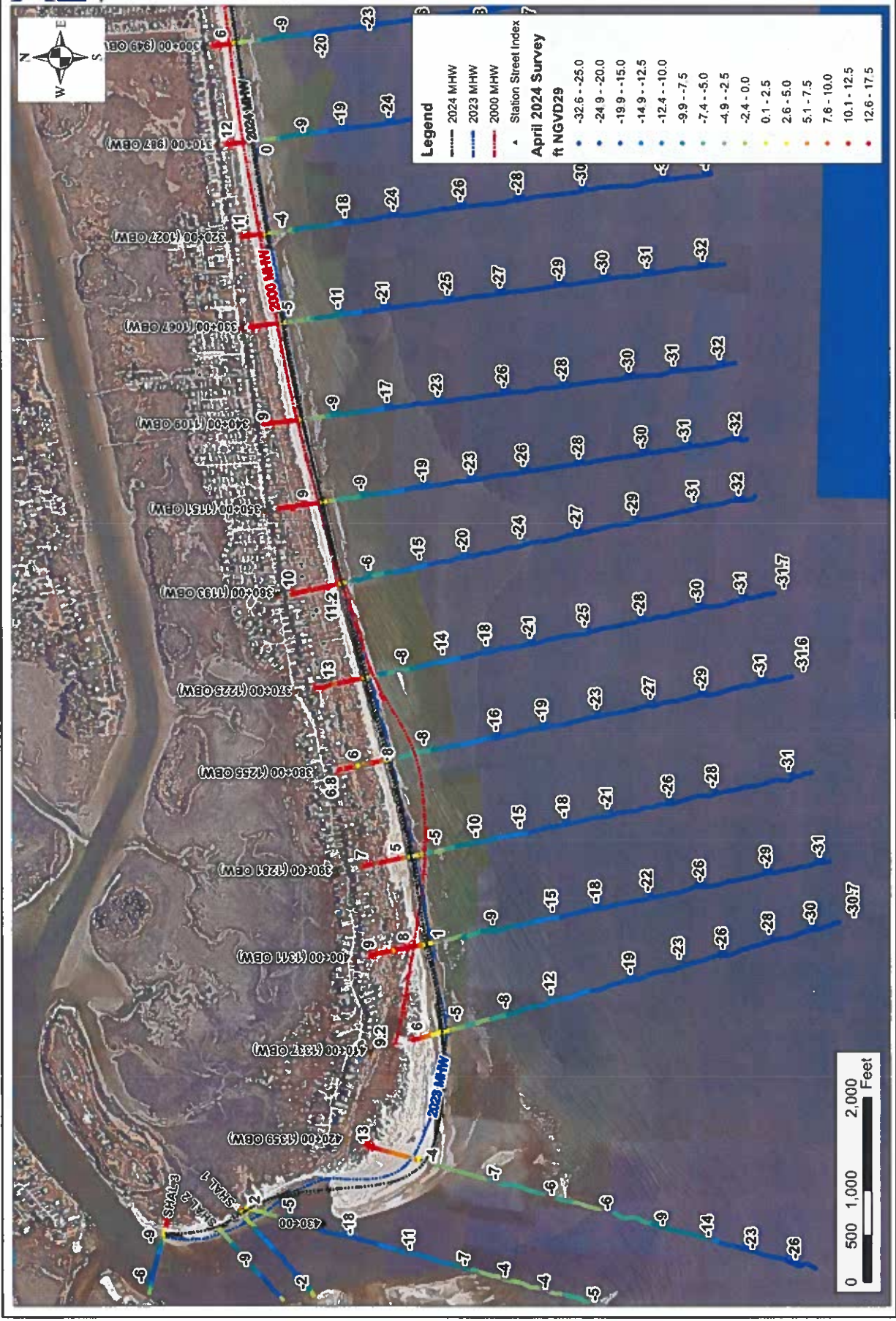
FIGURE B-4 2024 Survey Data and Established Monitoring Stations Shown. 2024 Mean High Water (MHW) Shoreline, 2023 MHW Shoreline, and 2000 MHW Shoreline. High-Resolution Aerial Imagery from Nearmap.com (January 2024).
