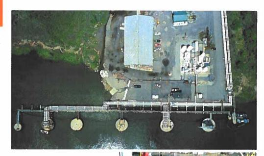
MidAtlantic was contracted directly with Kinder Morgan to perform a routine level above and underwater inspection of the CTR Dock at Kinder Morgan. The Project involved Level I and Level II/III inspection efforts on steel cellular mooring structures, steel pile pipe racks and stone gabion basket shoreline.
