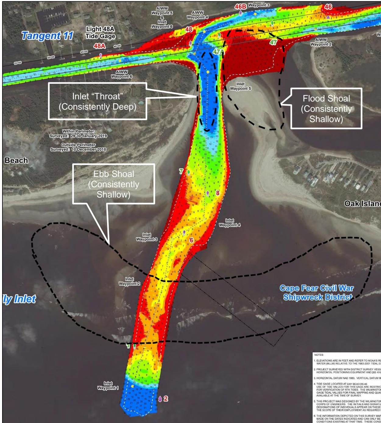
**Figure 1-4. Inlet Throat, Flood Shoal and Ebb Shoal at LWF Inlet
