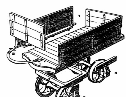
Assemble sides and ends to floor using liquid cement. Note that the notch in the centre of the ends is adjacent to floor and facing outwards.
