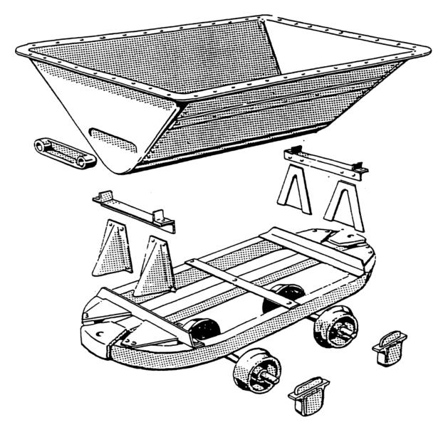
Wheels are a tight fit on the axles. They do not require any adhesive to secure them. For 32mm track wheels should be 28mm back to back.
