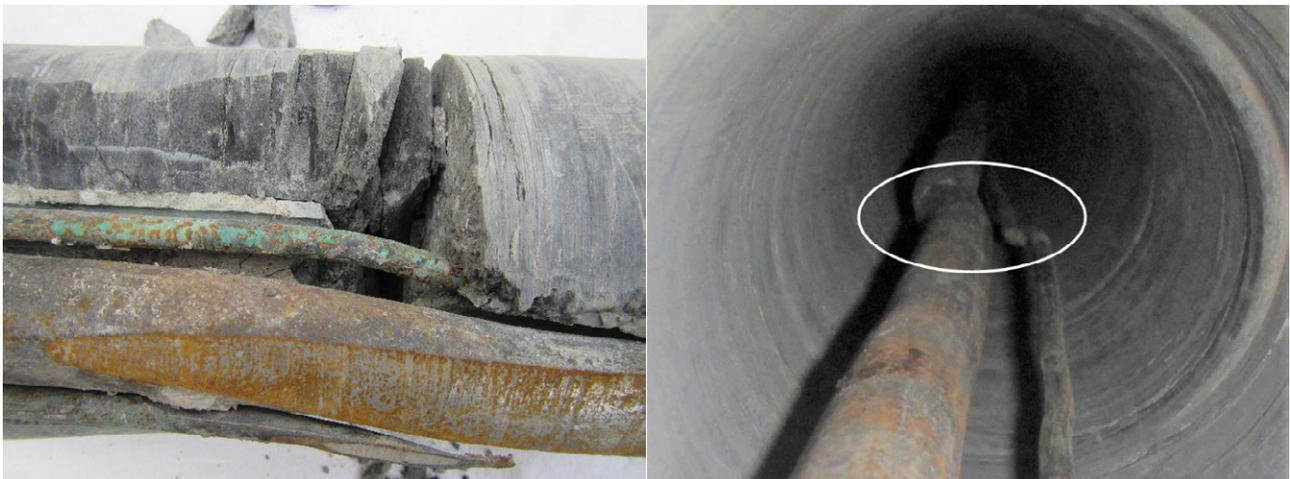
**Figure 19: Deformation of grouted and ungrouted rock bolts in the cavern roof observed after overcoring**
