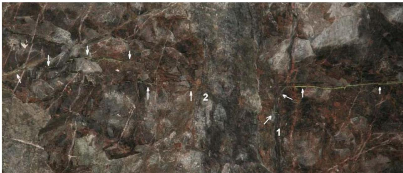
Figure 5 Hydraulic fracture (traceable via green proppant) exposed in drive (Jeffrey et al. 2009)
