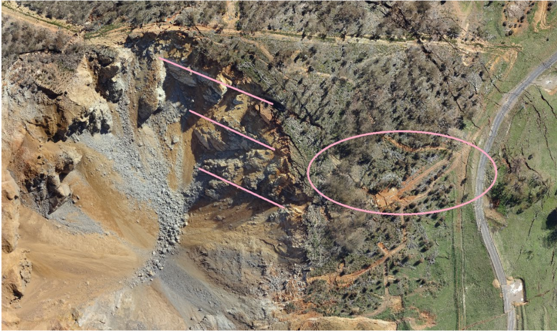
Figure 2 Predominant discontinuity orientation and impact of surface cracking beyond the crater limits
