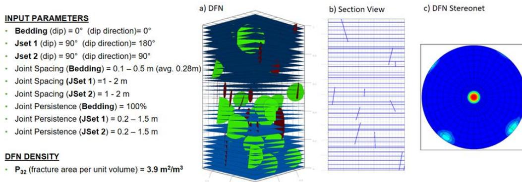
Figure 3. Discrete fracture network (DFN) to represent the Melbourne Formation siltstone
