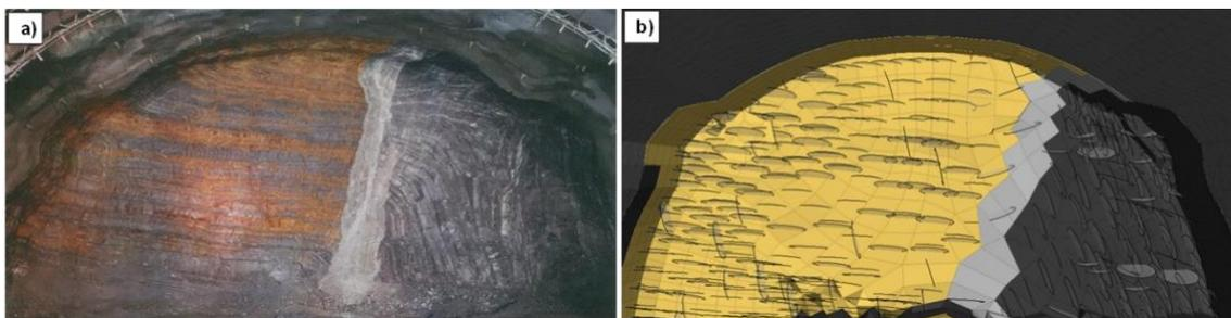
Figure 8. (a) Photograph of excavated face, (b) FLAC3D central tunnel (top heading) model geometry (disks showing ubiquitous joint orientation).
