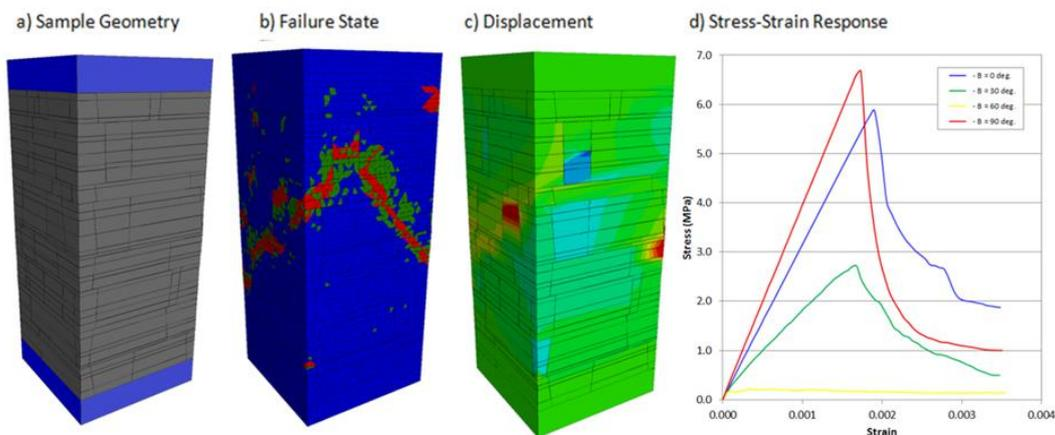
Figure 4. 3DEC model of simulated Melbourne Formation,  $\beta = 0$ ,  $\sigma_3 = 0$  MPa
