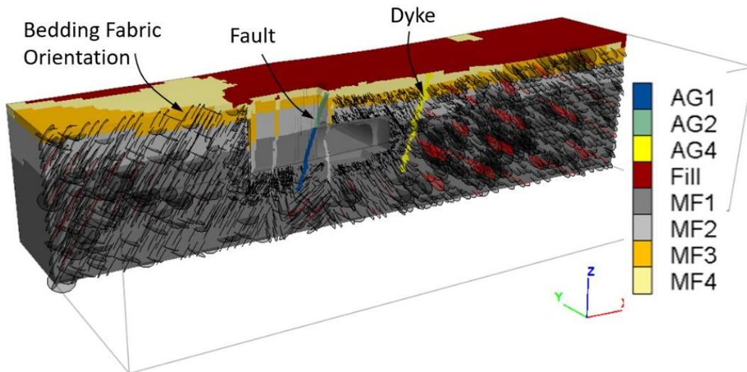
Figure 7. Geotechnical domains, major structures and bedding fabric simulated with the FLAC3D model.
