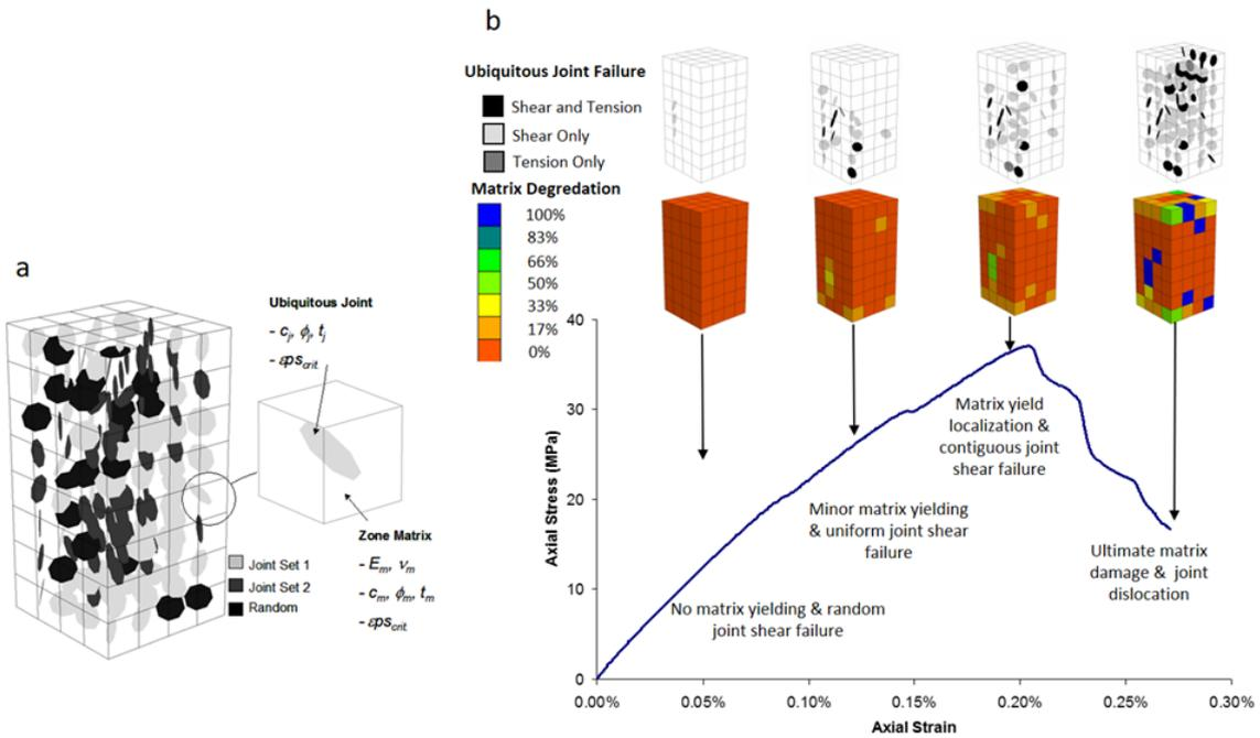
Figure 2. (a) Ubiquitous joint model: matrix and joint properties, (b) stress-strain response of simulated ubiquitous joint rock mass (Sainsbury et al, 2008)
