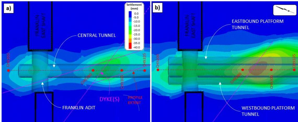
Figure 9. Estimated settlement (a) central tunnel and (b) trinocular cavern
