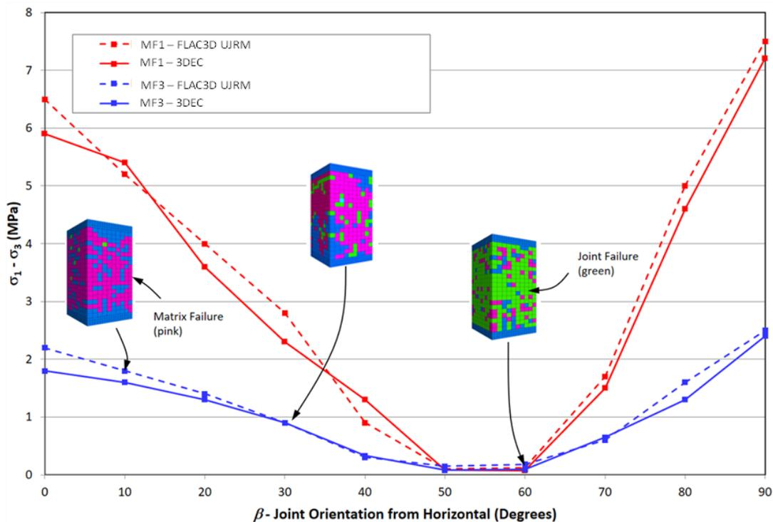
Figure 5. Calibrated UJRM anisotropic strength response compared to the discontinuum anisotropic response for Melbourne Formation
