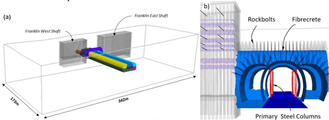
Figure 6. a) FLAC3D model geometry of the northern end of the State Library Station
