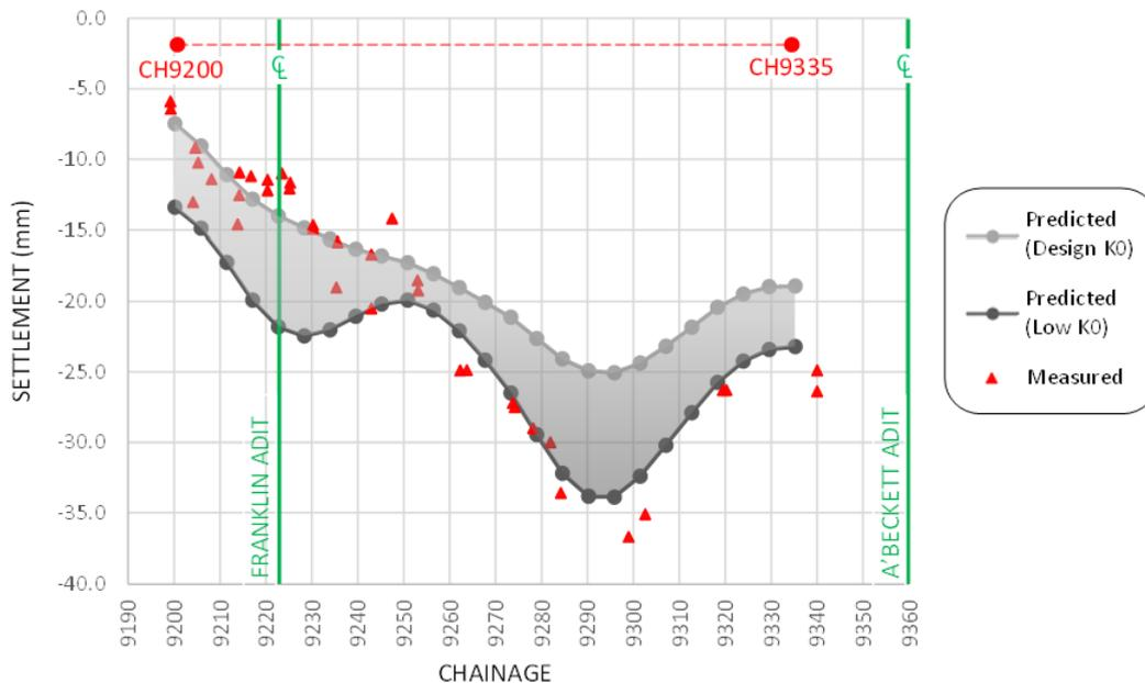
Figure 10. Calibration of predicted versus measured settlement for trinocular cavern
