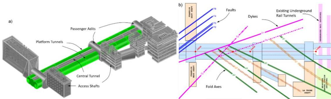
Figure 1. a) State Library Station configuration; b) Geological plan view showing major structures
