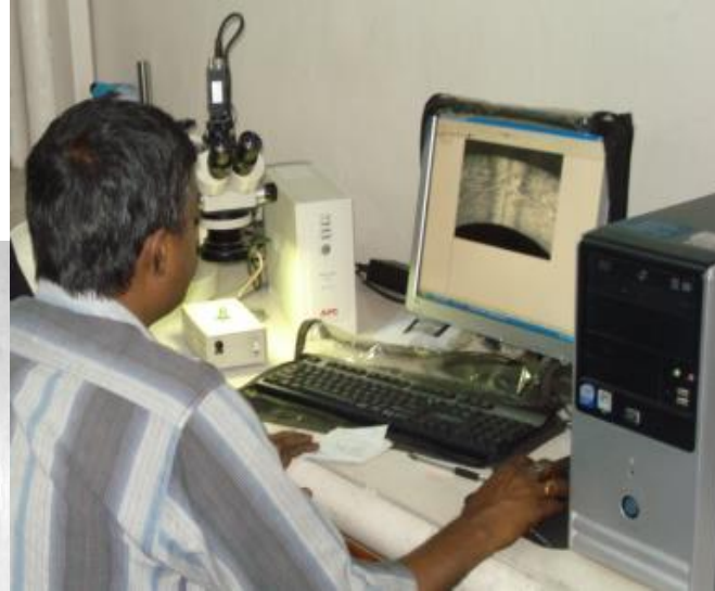
In-situ Weld Macro Examination facility using Metallurgical Microscope at Express Lab.
