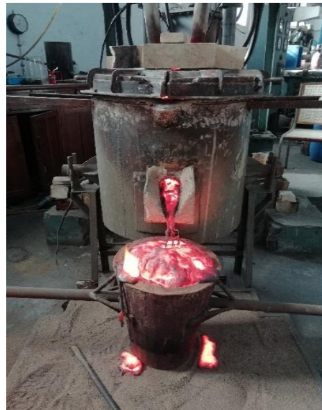
Silicothermic reduction in 50 kVA EAF
