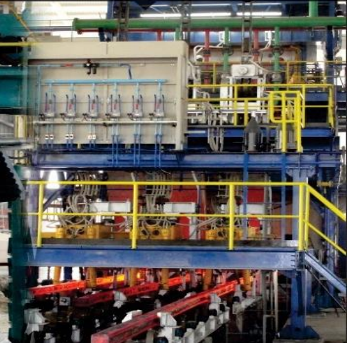
Continuous Casting Machine
