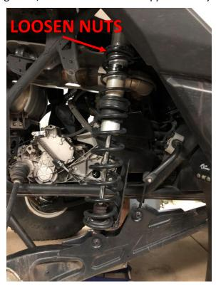
5. Now the passenger side limit strap can be installed. Remove the passenger side upper shock nut and bolt and replace them with the supplied hardware as shown below. Snug tighten the nut for now. NOTE: The new shorter bolt goes in the top shock mount and the new longer bolt goes in the bottom shock mount.
