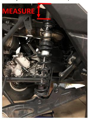
4. Remove the passenger side coil spring tension by loosening both jam nuts on top of the coil spring. To loosen these nuts, first spin the top nut counterclockwise (top looking down) with the Can-Am supplied tool that came with your vehicle. Then loosen the nut directly below that one. The coil springs should now be loose. By spinning them, move the two nuts to approximately 4" above their original position.
