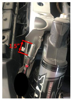
15. With the front tires of the vehicle still in the air, measure the distance between the center of the bottom shock bolt and the clevis limit strap mounting hole. Write down this value. The value should be around 23.5". If it is not, adjust the clevis position to make this dimension 23.5".
