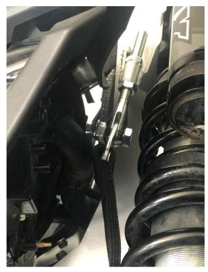
18. Slowly lower the floor jack allowing the new limit strap to hold the suspension up. Wiggle the limit strap bottom mounting bracket so that it is pointing at the top shock bolt if not already.
