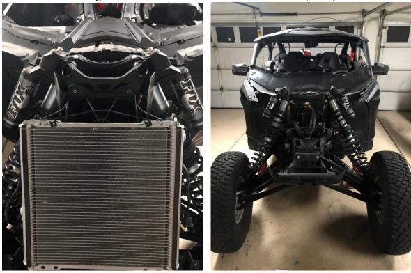
3. Securely raise the front of the vehicle until the two front tires are about ¼" off the ground. Use jack stands on the vehicle frame for safety. Remove the top shock bolts and rest the top of the shocks beside the top shock mount (frame).
