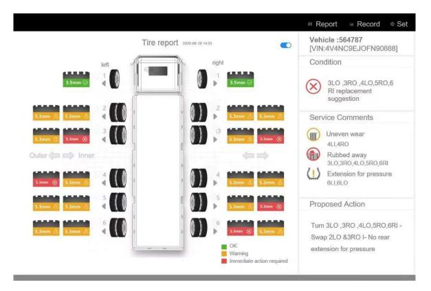
The software-based report shows issues with tires, marks them up on a diagram, and provides recommendations such as tire rotation or replacement.
