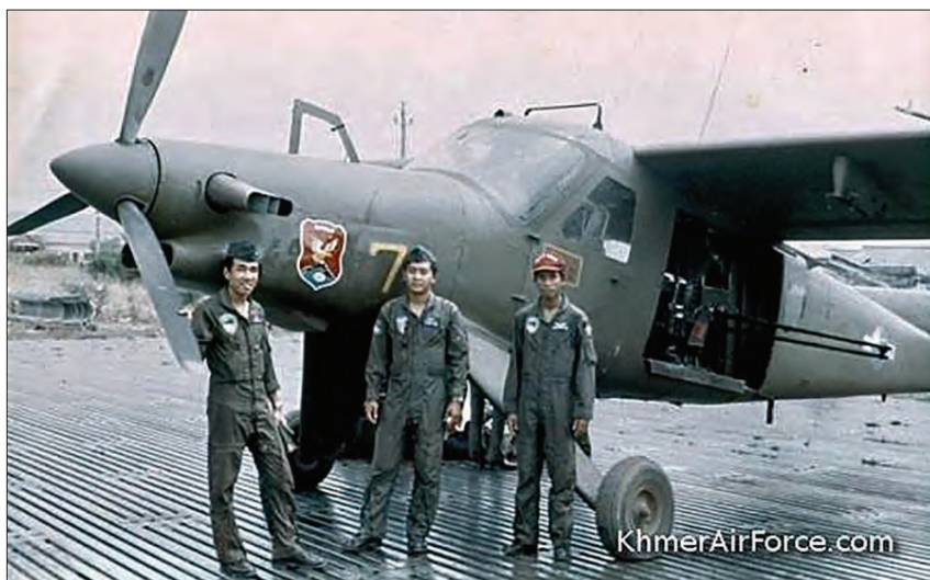
KAF crew by their AU-24 Helio Stallion Short Takeoff and Landing (STOL) aircraft. The USAF provided fifteen of these gunship versions to the KAF in 1972.
