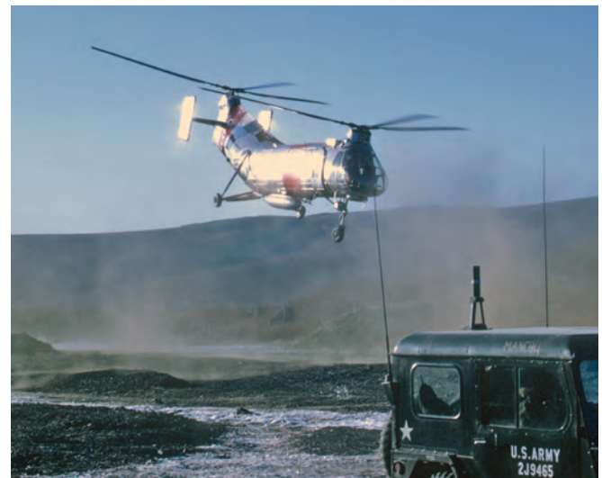
H-21 “Flying Banana” supporting Army operations in Alaska. Built by Boeing/Vertol, it was a famous Piasecki design and was heavily used by both Air Force and Army. This model had a folding hoist over the door just aft of the cockpit windows, used for lifting survivors during a hover pickup.
