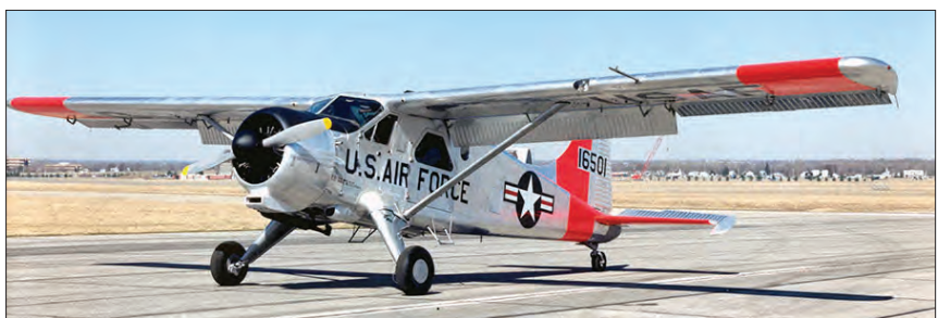
The Canadian-built de Havilland "Beaver." This workhorse was designed for operations in extremely cold climates. Designated "U-6" by the U.S. Army, the Beaver was one of the most useful utility aircraft in the Air Force. It had excellent STOL performance and could carry six passengers or just over a ton of cargo.
