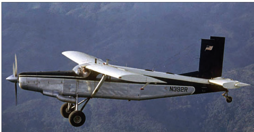
The Swiss-built turbine powered Porter can carry up to 10 passengers or over 2600 pounds of cargo and take off in less than 700 feet, making it very useful in the jagged karst mountains of Laos.
