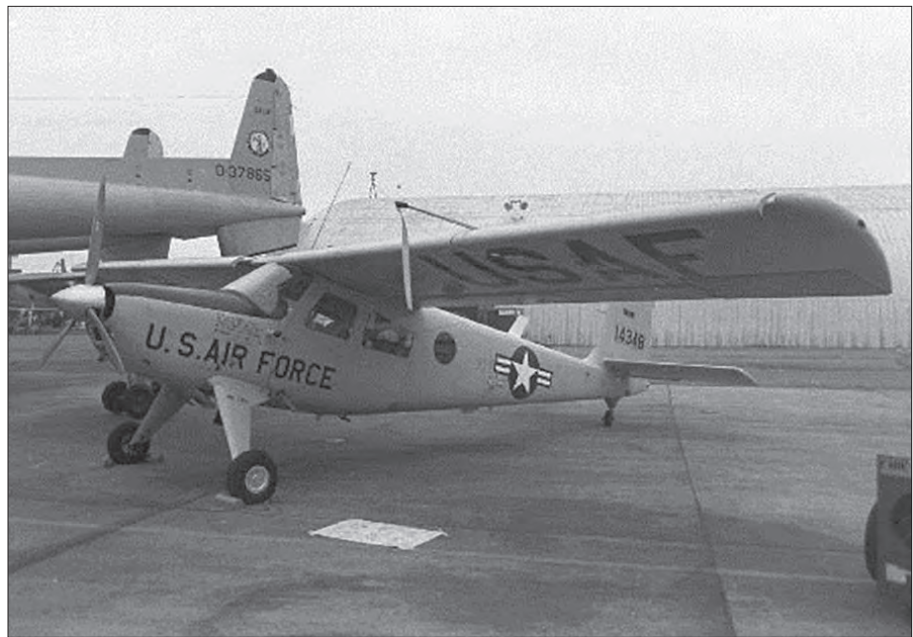
The U-10 “Super Courier,” by Helio Aircraft Company, in Kansas, can take off in less than 200 feet, carry 5 passengers or 1300 pounds, and is controllable down to 28 knots! Max range is over 1000 miles.
