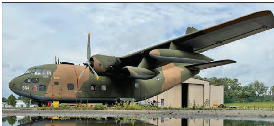
The Fairchild C-123, developed from a Chase glider design and boosted by auxiliary jet engines. Main power was two reversed Pratt & Whitney R-2800 recip engines.
