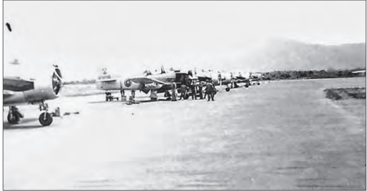
Royal Lao Air Force AT-28s. This was the fighter conversion of USAF T-28 trainers.
