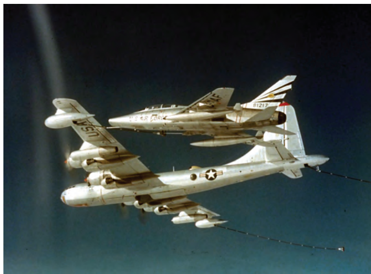
KB-50J refueling an F-100 fighter. The red stripe around the tail cone of the left J-47 is where the white-hot turbine spins. Note that it is in line with the front of the wing flaps, where five fuel lines are. Just ahead of the star insignia is the “blister” where Webster saw the tailcone separate and the inner left wing instantly erupt in flames that went past the tail and melted the plastic of his blister. USAF photo.
