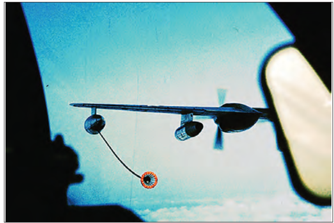
Receiver pilot's view of the "basket" and hose deployed by the KB-50J. The jet engine shown is the counterpart of the engine that blew apart and sprayed the flap "well" with very hot pieces of the failed turbine at the rear of the J-47 engine.
