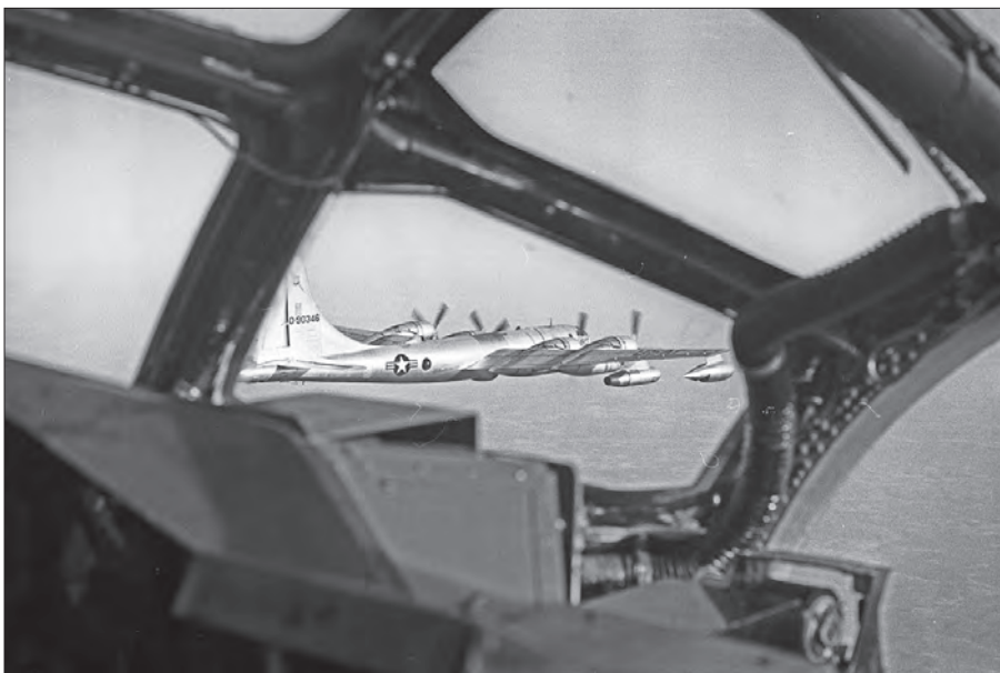
View of lead tanker in formation. Aft exit door is aft of the star insignia. View is from the co-pilot's seat on the right side of the cockpit. The top of the aircraft commander's instrument panel is in the foreground. In the original bomber configuration the bombardier's position would be at the right, in the cockpit nose window. Photo: author.
