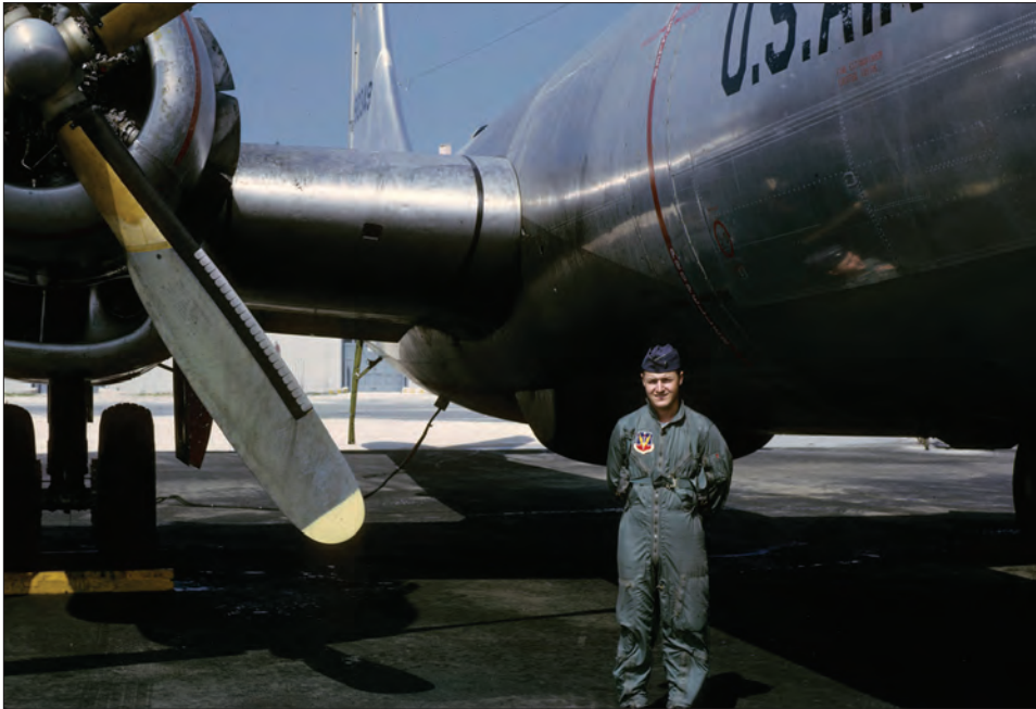
Tilton next to the fuselage of a KB-50J on his first TDY to Bermuda, not yet checked out nor even on a crew, and still a 2nd lieutenant, in May of 1963. The 18-foot diameter propellers were optimized for high-altitude operation and did not allow full power (60" Hg, 2500rpm, 3500 HP from 4,360 cu) to be developed on the runway until the plane reached 100 knots airspeed.
