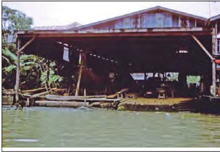
You can still see the prow of a rice barge under construction in this boat house. No longer visible are builders cutting hull planks with two-man crosscut saws.
