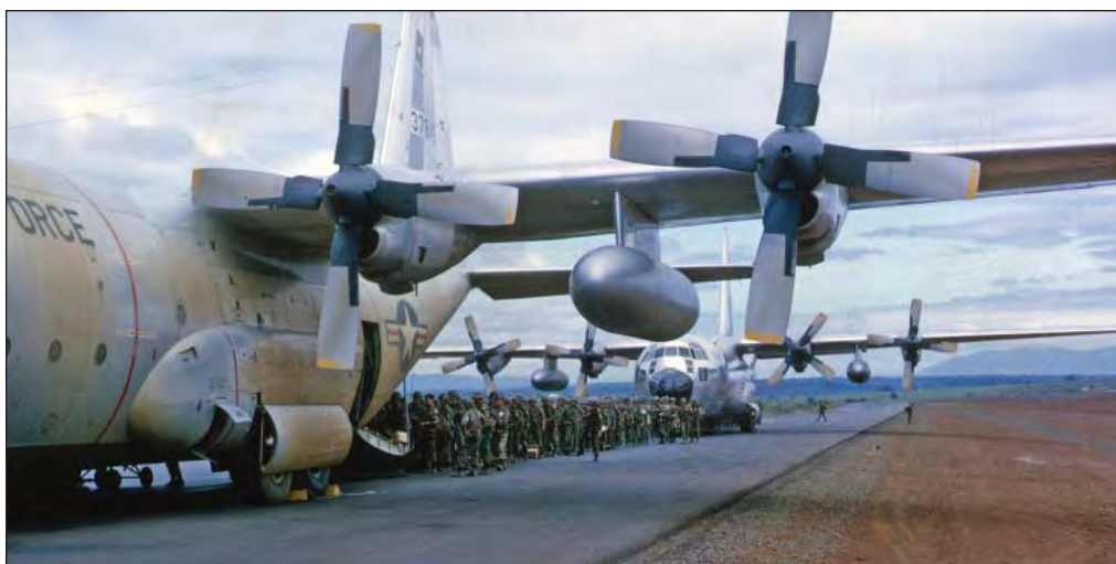
ARVN (South Vietnamese Army) troops loading onto a C-130E. Note the huge auxiliary fuel tanks, which enabled the C-130 to make very long over-water hops. The ARVN loaded 300 troops onto a C-130, which would carry 55 or 60 U.S. troops in combat gear. The soldiers had to stand up for the flight. Photo by Jimmy Honeycutt.
