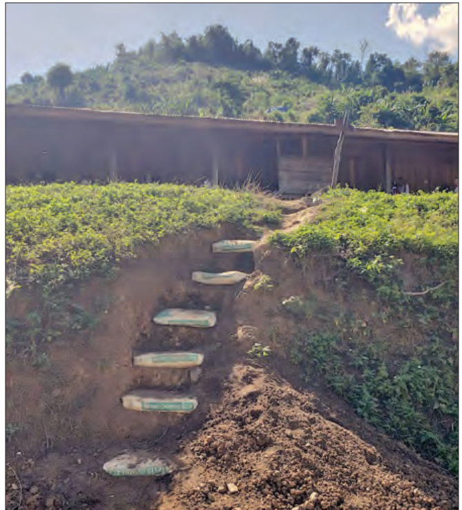
Because there was flooding at SopOr before this concrete could be used, it hardened in the bags, which were put to use as makeshift steps anyway.
