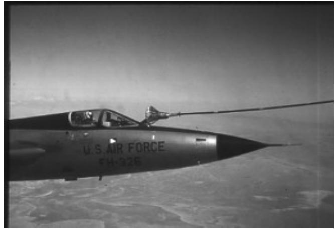
F-105 hooked up and taking fuel from the left reel of a KB-50J over the Mississippi River, 1963,
